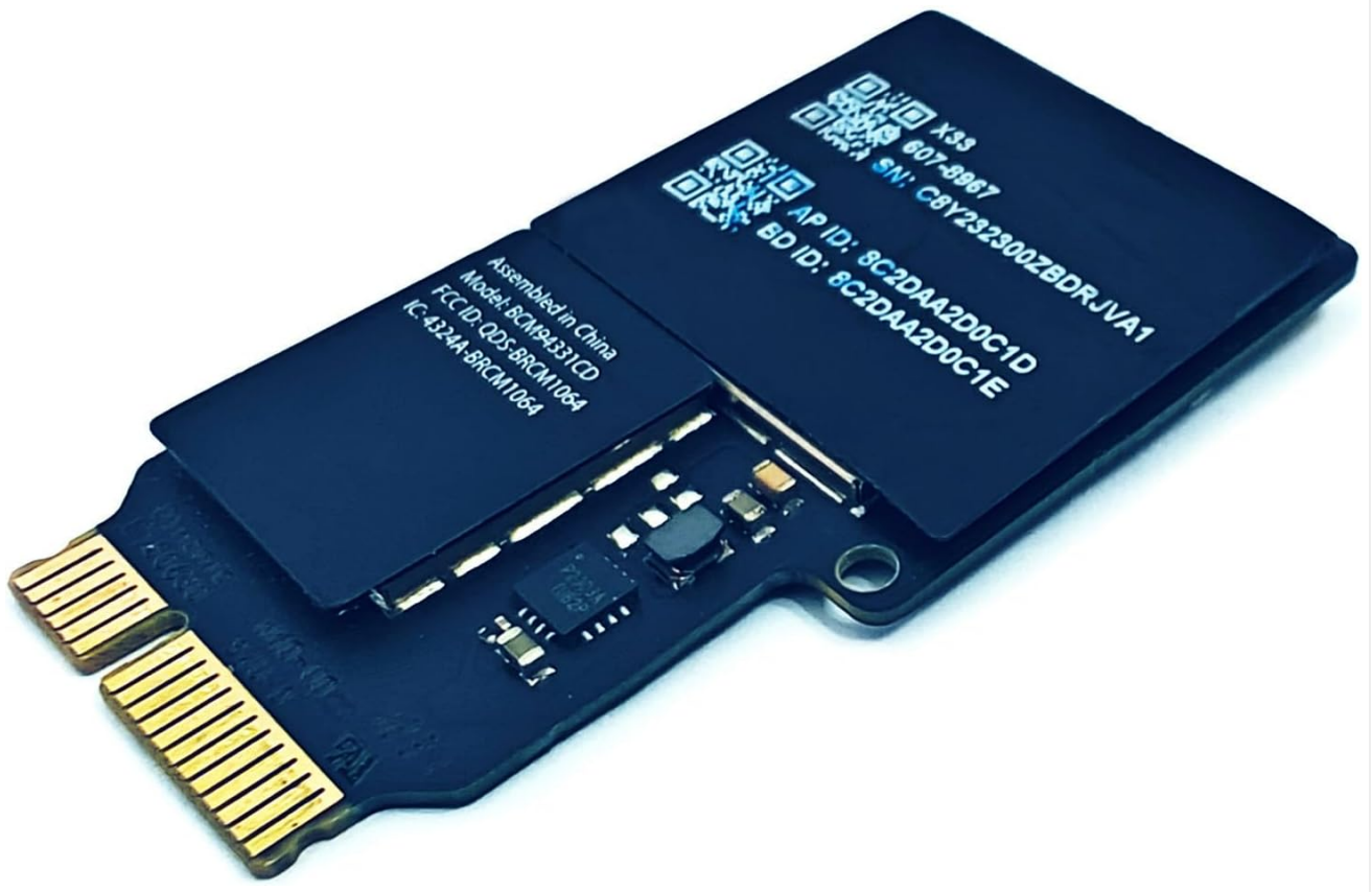
Figure 2.1: Front view of the Nockchawon BCM94331CD Bluetooth and Wi-Fi Airport Card. This image displays the front side of the Nockchawon BCM94331CD wireless card, showing the gold-plated connector pins and the main chip components. The card features labels for its model number and regulatory information.
