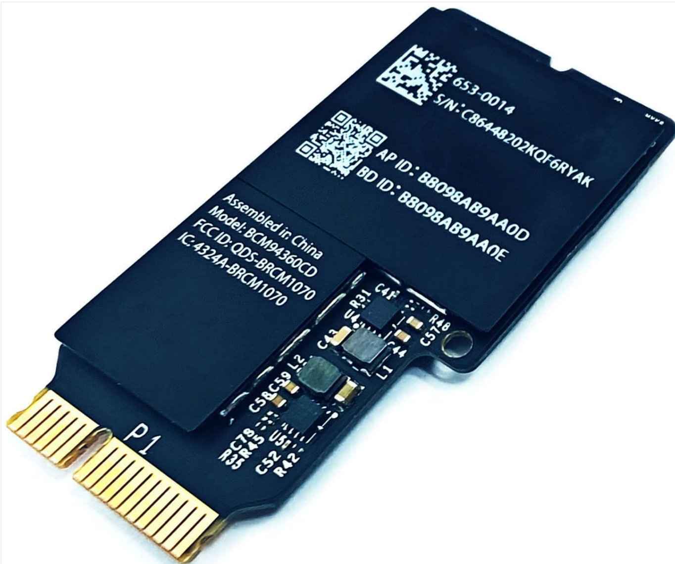
Figure 2.1: Front view of the Nockchawon BCM94360CD WiFi Bluetooth Airport Wireless Card. This image displays the front side of the BCM94360CD wireless card, showing its primary components and the gold-plated connector pins. Key identifying numbers such as BCM94360CD and 653-0014 are visible.
