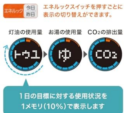
Figure 1: Noritz RC-J101E Kitchen Remote Control Display. This image shows the main kitchen remote display, highlighting the Enerlook function with blue and orange indicators for energy usage and CO 2 emissions. It also displays current time and temperature settings.
