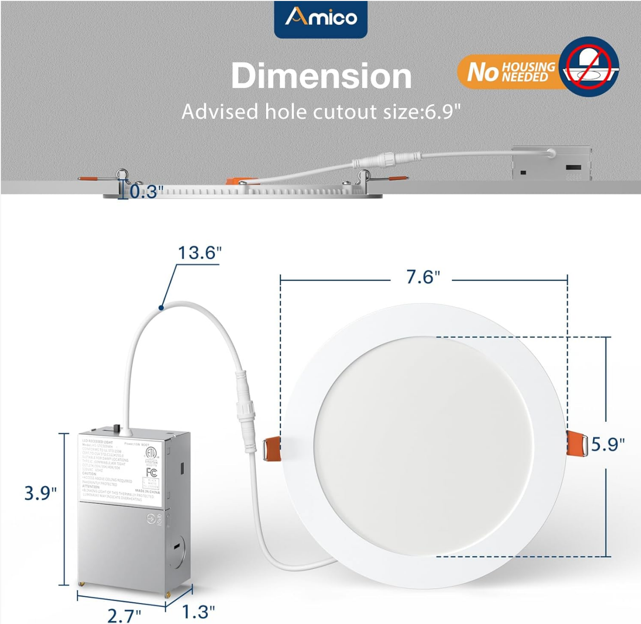
Image: Detailed dimensions of the Amico 7-inch LED Recessed Light and its junction box. The advised hole cutout size is 6.9 inches.
