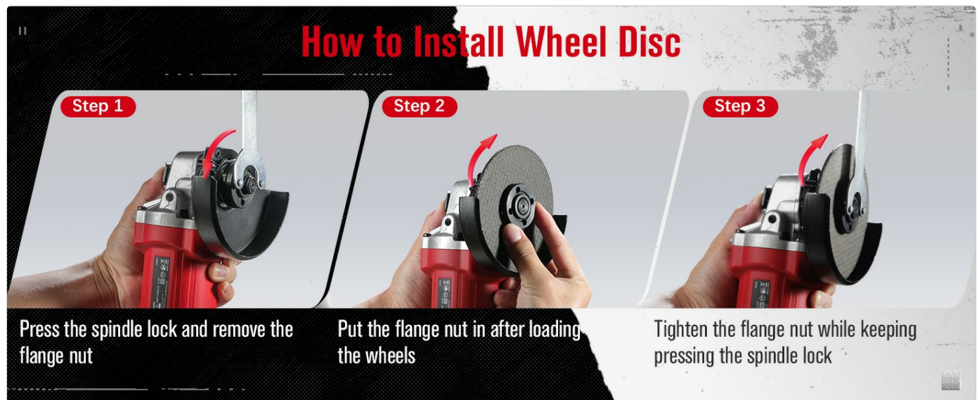
Image: Step-by-step visual guide for installing a wheel disc on the angle grinder, detailing the use of the spindle lock and flange nut wrench.
