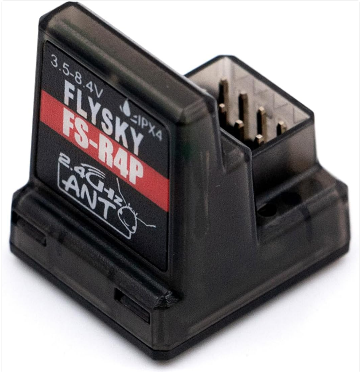
Figure 5: Close-up view of the FS-R4P receiver's pin connectors. This image clearly shows the PWM output pins, indicating where to connect servos and other components for proper functionality.
