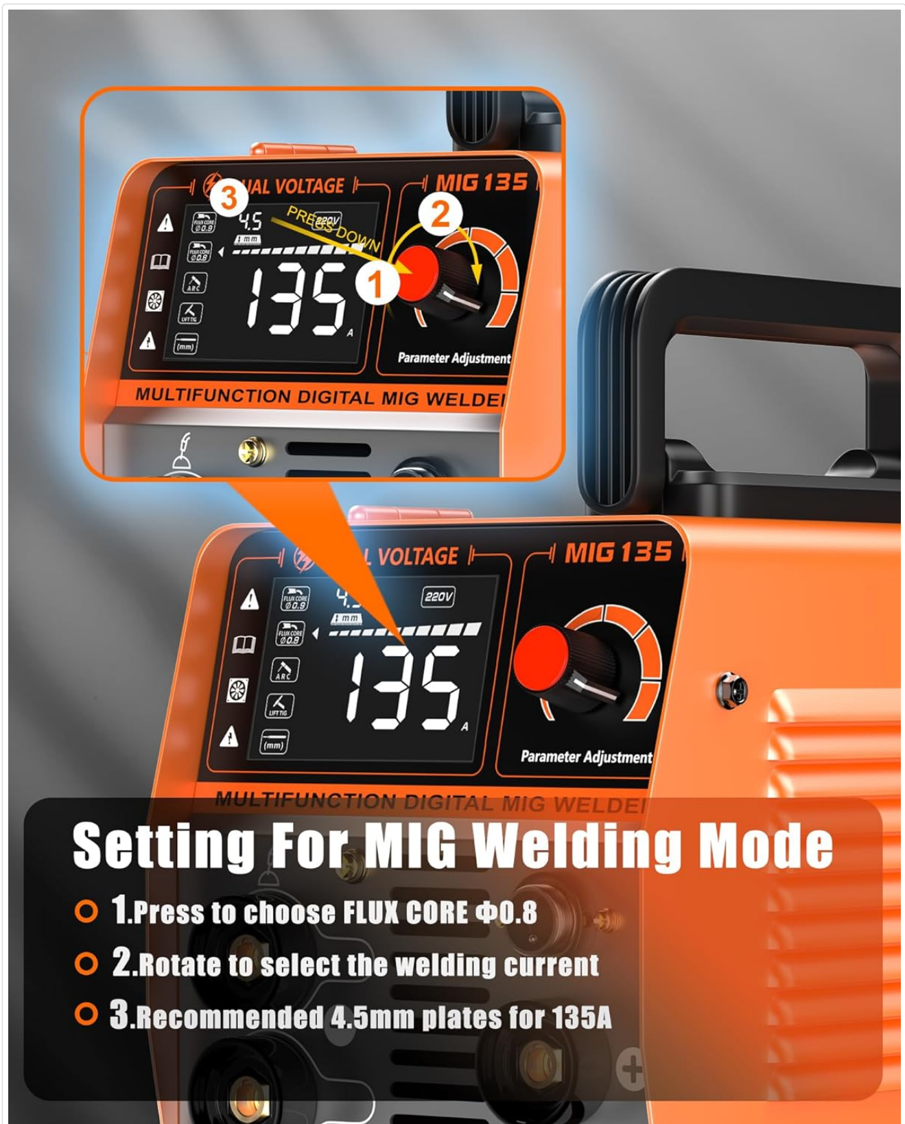
Image: The control panel displaying settings for MIG welding mode. It shows pressing to choose FLUX CORE \Phi 0.8, rotating to select welding current, and a recommendation of 4.5mm plates for 135A output.
