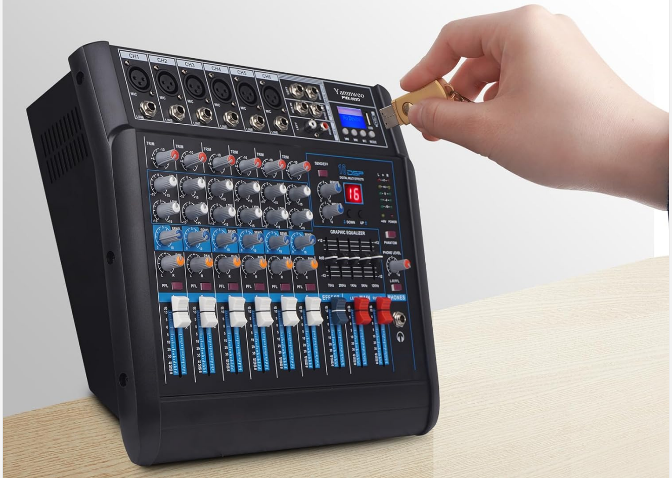
Figure 2: Illustrates connecting a USB disk to the dedicated USB slot on the mixer for direct audio playback.
