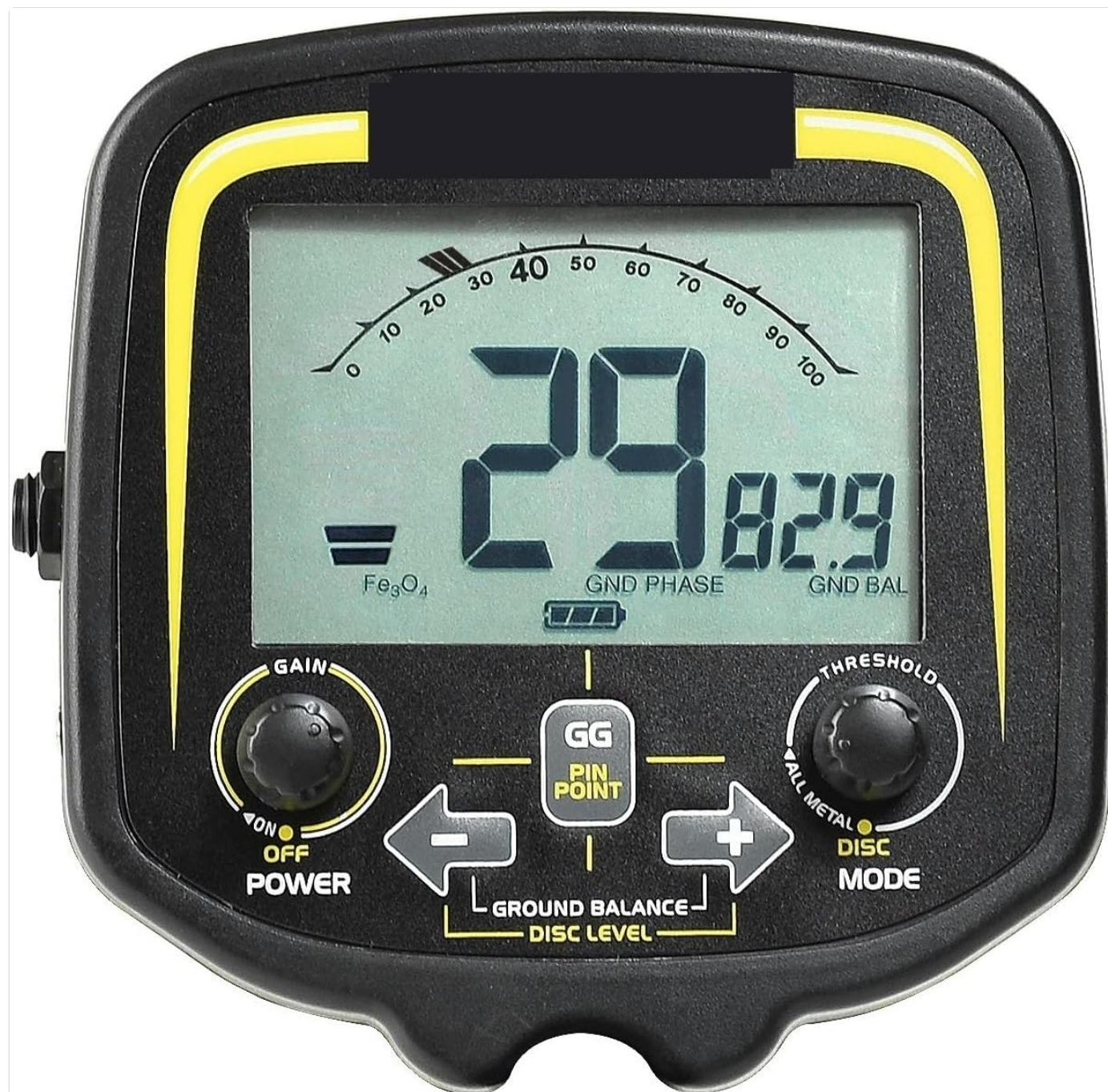
Figure 3: Control Panel and LCD Display. This image highlights the detector's control panel, including the POWER/GAIN knob, THRESHOLD/ALL METAL/DISC MODE knob, GROUND BALANCE buttons, and the LCD screen displaying target ID, depth, and battery status.
