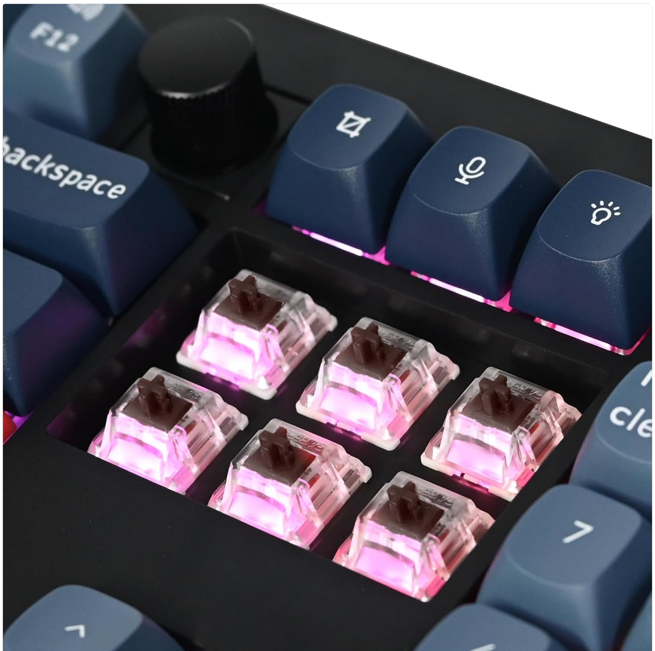
Image: Close-up view of the keyboard with several keycaps removed, showing the hot-swappable switch sockets and a Gateron Jupiter Brown switch.
