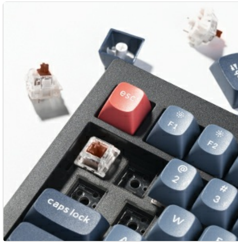
Image: A close-up of a keycap and switch being removed from the keyboard, demonstrating the hot-swappable feature.
