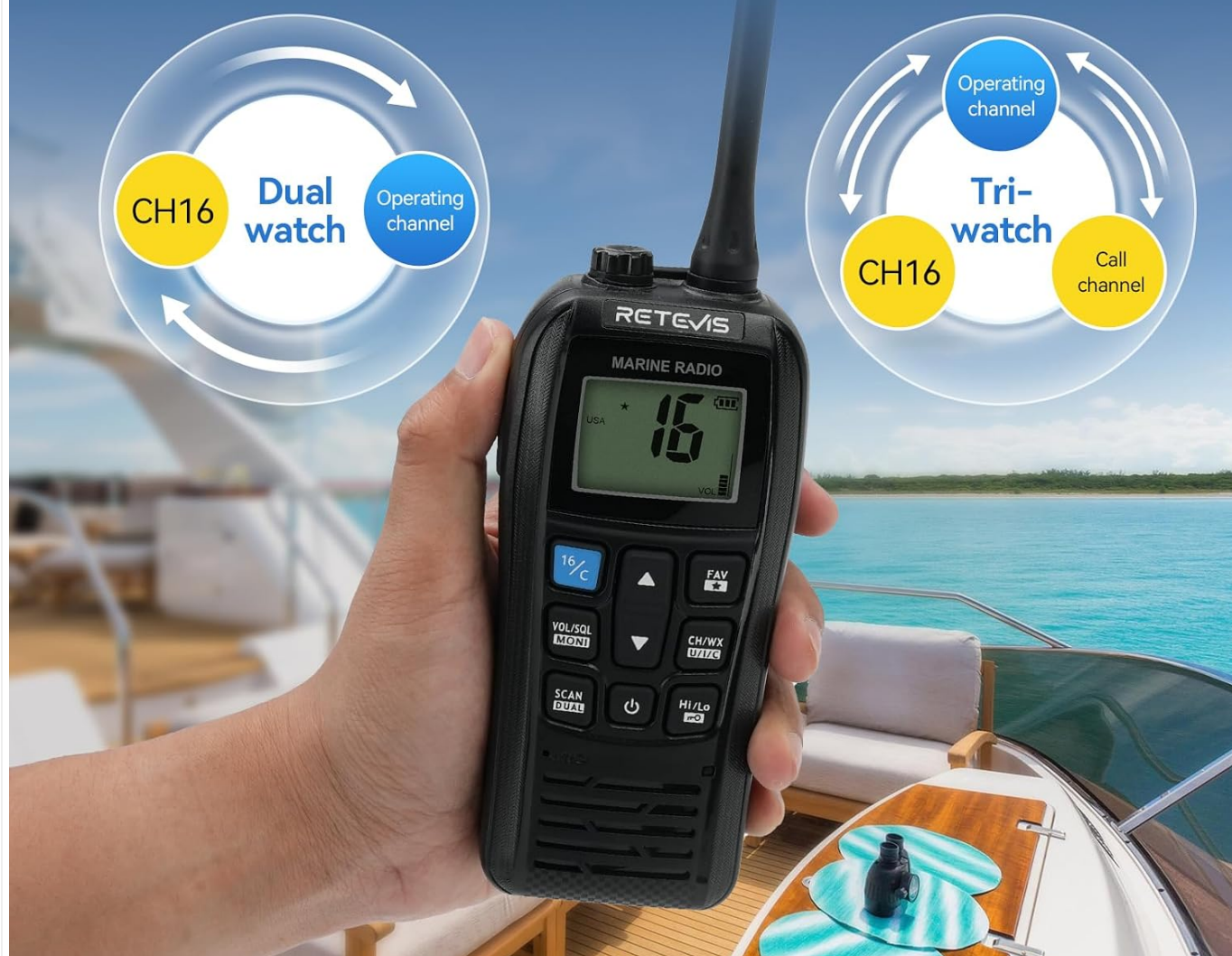
Figure 4.2: Dual Watch and Tri-watch modes for monitoring multiple channels.
