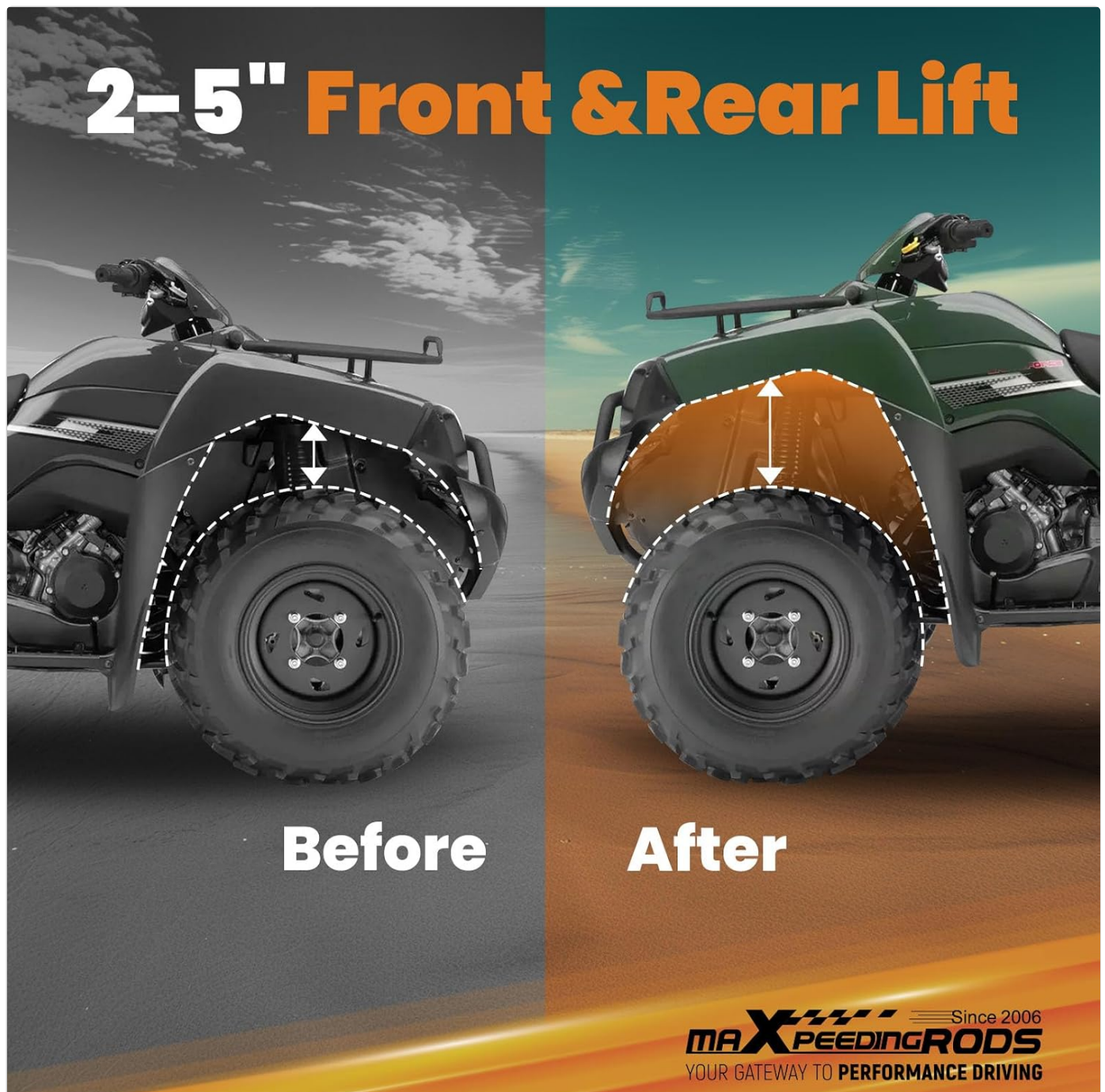
Image: A side-by-side comparison of an ATV, illustrating the increase in ground clearance after the installation of a 2-5 inch lift kit.
