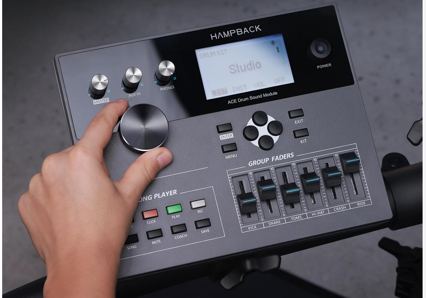
Figure 3.5: The HAMPBACK ACE-360 sound module. This module provides access to 918 sounds, 52+20 drum kits, and 15 demo songs.
