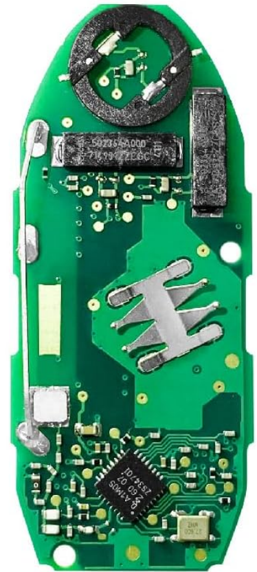
Image: Internal components of the key fob, including the PCB board and chip, with frequency and chip type verification.
