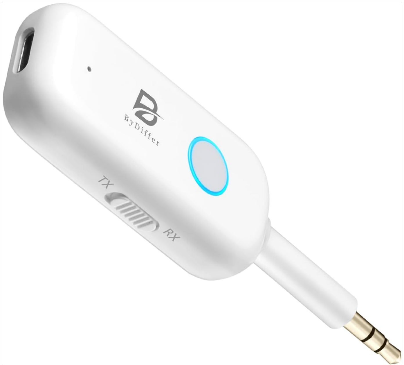
Image 1: Front view of the BYDIFFER Bluetooth Transmitter Receiver. This image displays the device's main features including the USB-C charging port, an LED indicator light, the central multi-function button, a slider switch for selecting Transmitter (TX) or Receiver (RX) mode, and the integrated 3.5mm audio jack.
