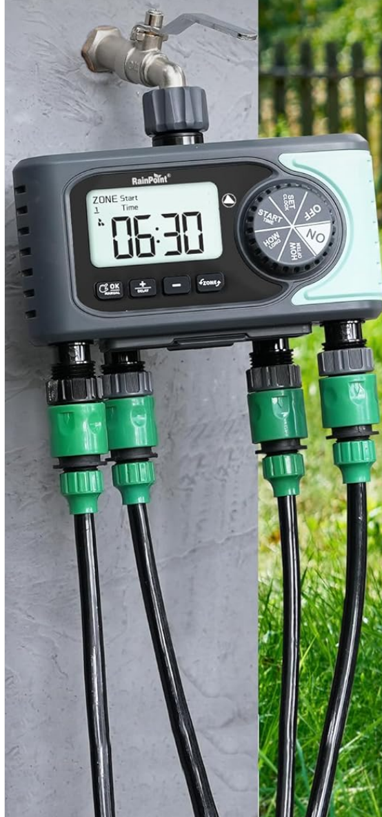
Figure 4: The timer's display showing options for setting watering cycle modes, including start time, duration, and frequency.
