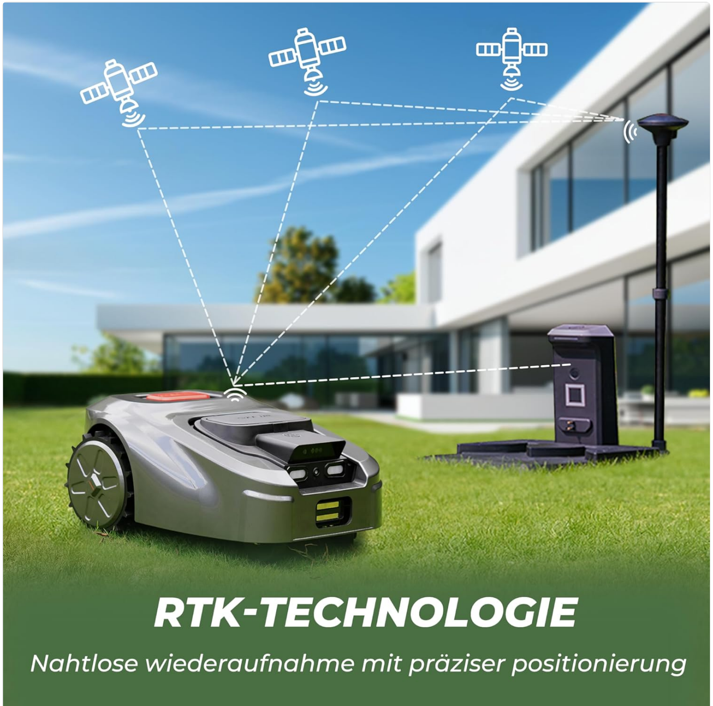
Figure 4.1: The RTK base station and robotic mower receiving positioning signals from satellites for accurate navigation.
