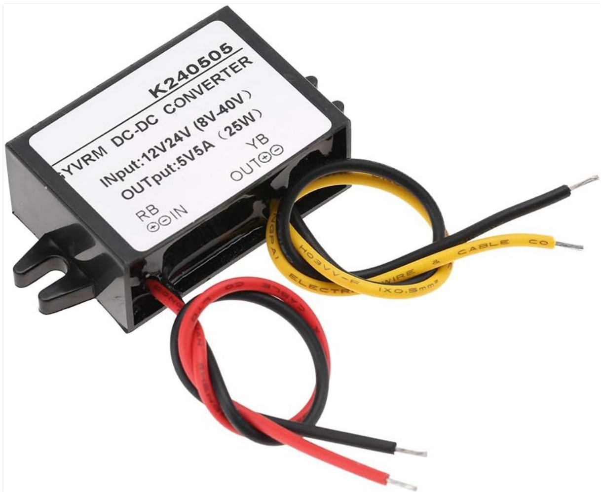
Figure 4: Input (red/black) and output (yellow/black) wiring connections.
