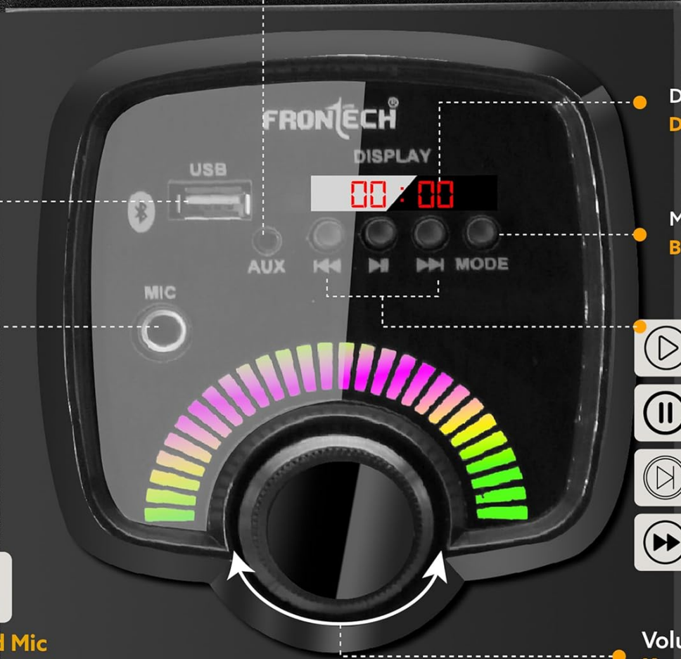
Figure 4.2: Close-up of the speaker's control panel, detailing the LED digital display, USB port, AUX input, mode selection, playback controls, volume knob, and microphone input.
