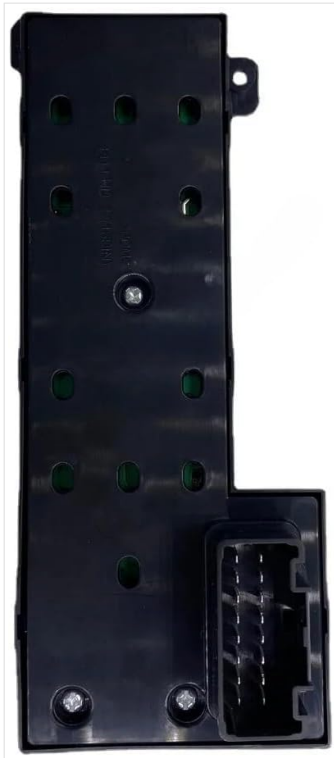
Figure 3: Rear view of the master window switch, highlighting the electrical connector ports that need to be properly connected during installation.
