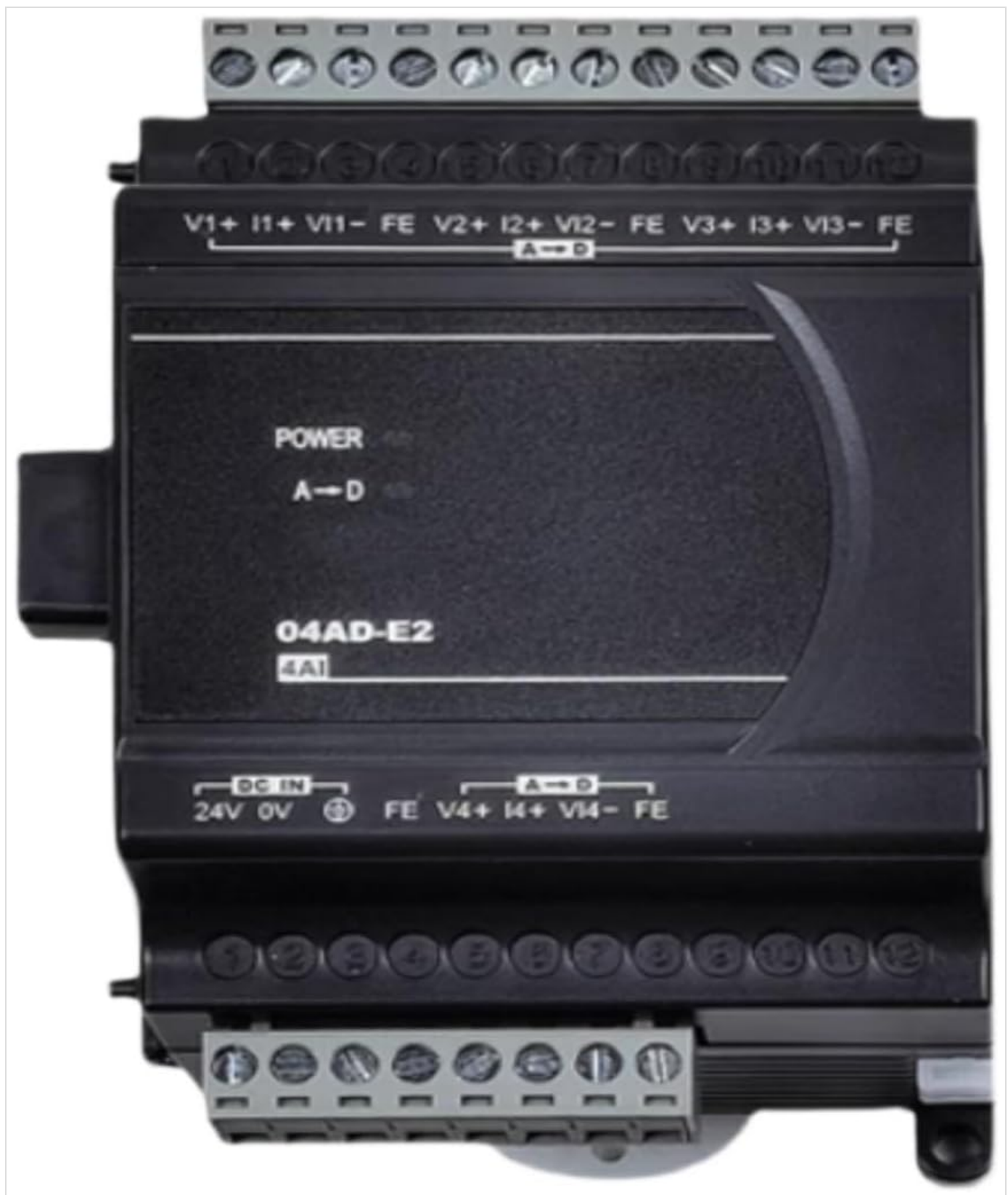
Figure 3.1: Representative image of a CEMELI E2 series PLC module. This specific image shows a DVP04AD-E2 (4 Analog Input) module. The DVP04PT-E2 module will have similar physical characteristics but is configured for RTD inputs. The module features multiple screw-terminal blocks for input/output connections at the top and bottom. The central panel includes indicators for 'POWER' and 'A->D' (Analog to Digital conversion). The top terminals are labeled V1+, I1+, VI1-, FE, V2+, I2+, VI2-, FE, V3+, I3+, VI3-, FE. The bottom terminals include DC IN 24V 0V, FE, V4+, I4+, VI4-, FE.
