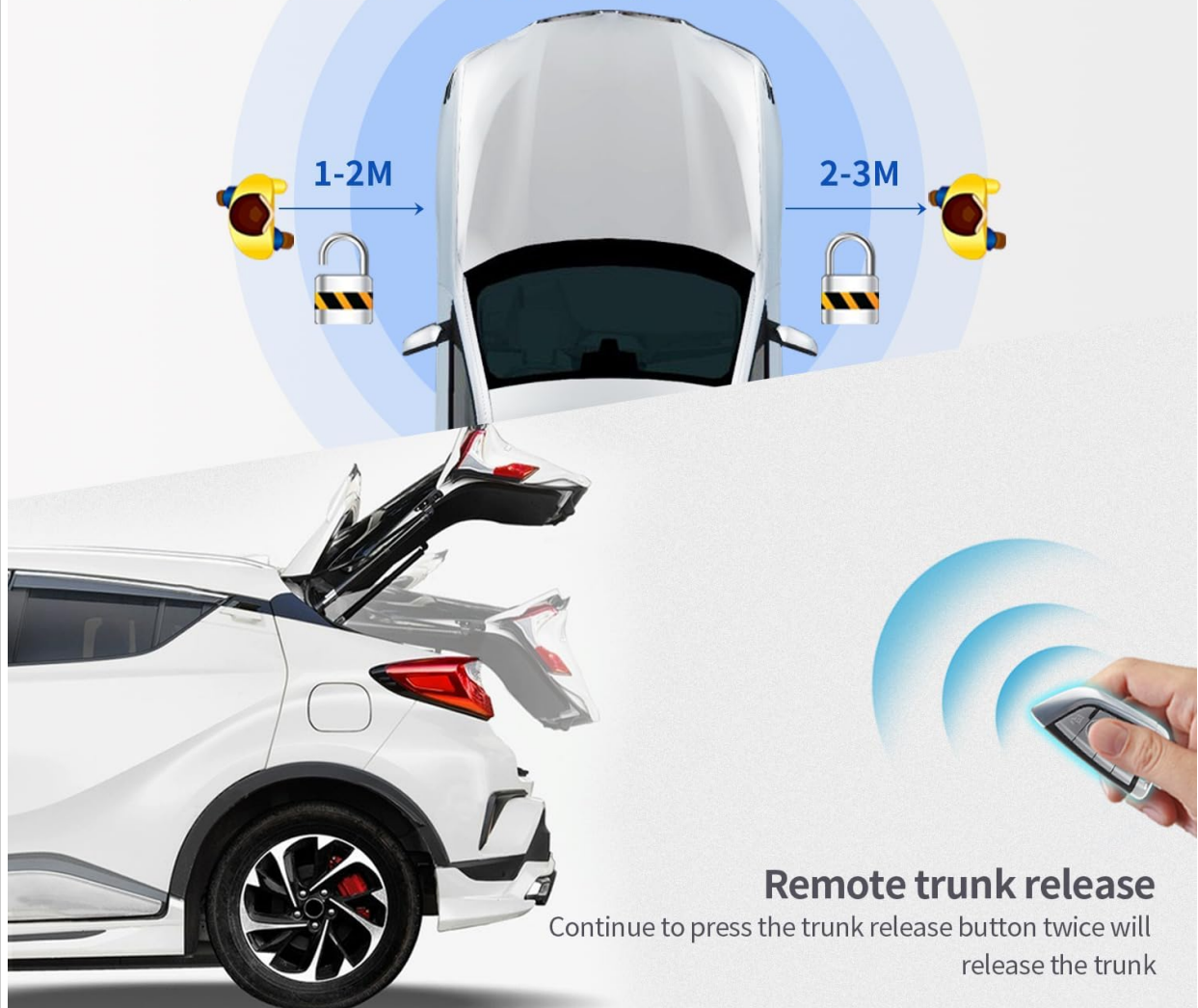
Figure 4: Visual representation of the PKE system's range for automatic locking and unlocking, along with the remote trunk release function.
