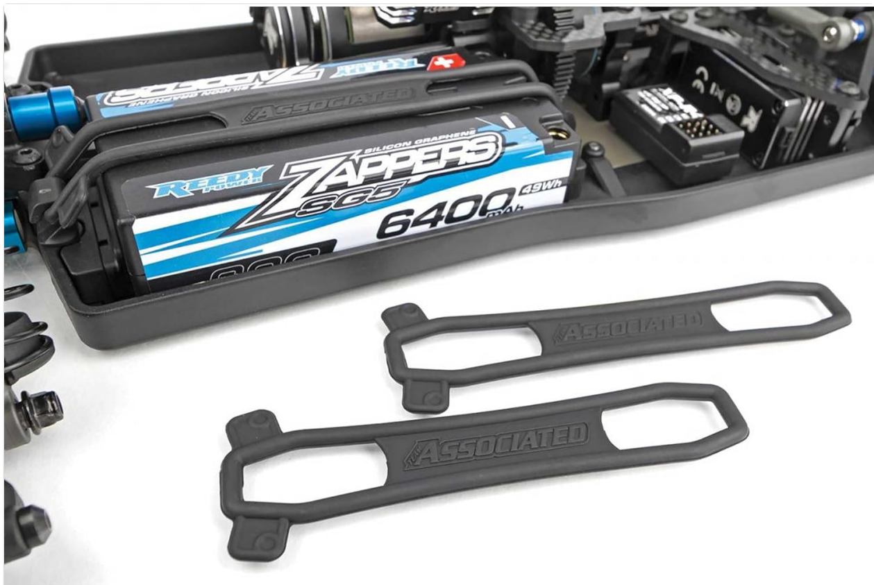
Image: The battery compartment showing a battery installed and the associated O-ring style hold-down straps.
