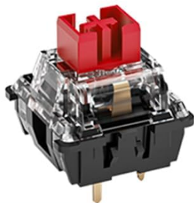
Figure 3: Diagram showing the components of a hot-swappable mechanical switch, emphasizing the ease of replacement without soldering. Specifications for the red switch are also shown: Actuation Force: 45g, Actuation Distance: 2.4mm, Travel Distance: 4.4mm.
