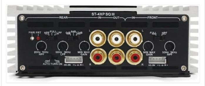
This image shows the input and control panel of the Zapco ST-4XP-SQ-III amplifier. Visible controls include gain adjustments, high-pass filter (HPF), low-pass filter (LPF), bass boost, and RCA input jacks for front and rear channels. Speaker level inputs and an auto-on switch are also present.
