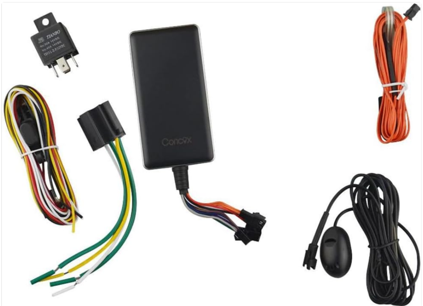
Figure 2: GT06N GPS Tracker and Accessories. This image shows the main GT06N tracker unit, a relay, a microphone, an SOS button, and various wiring harnesses, illustrating the complete package contents.
