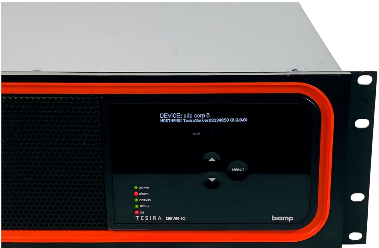
Figure 2.6: Front panel display showing operational status and device identification after successful boot.
