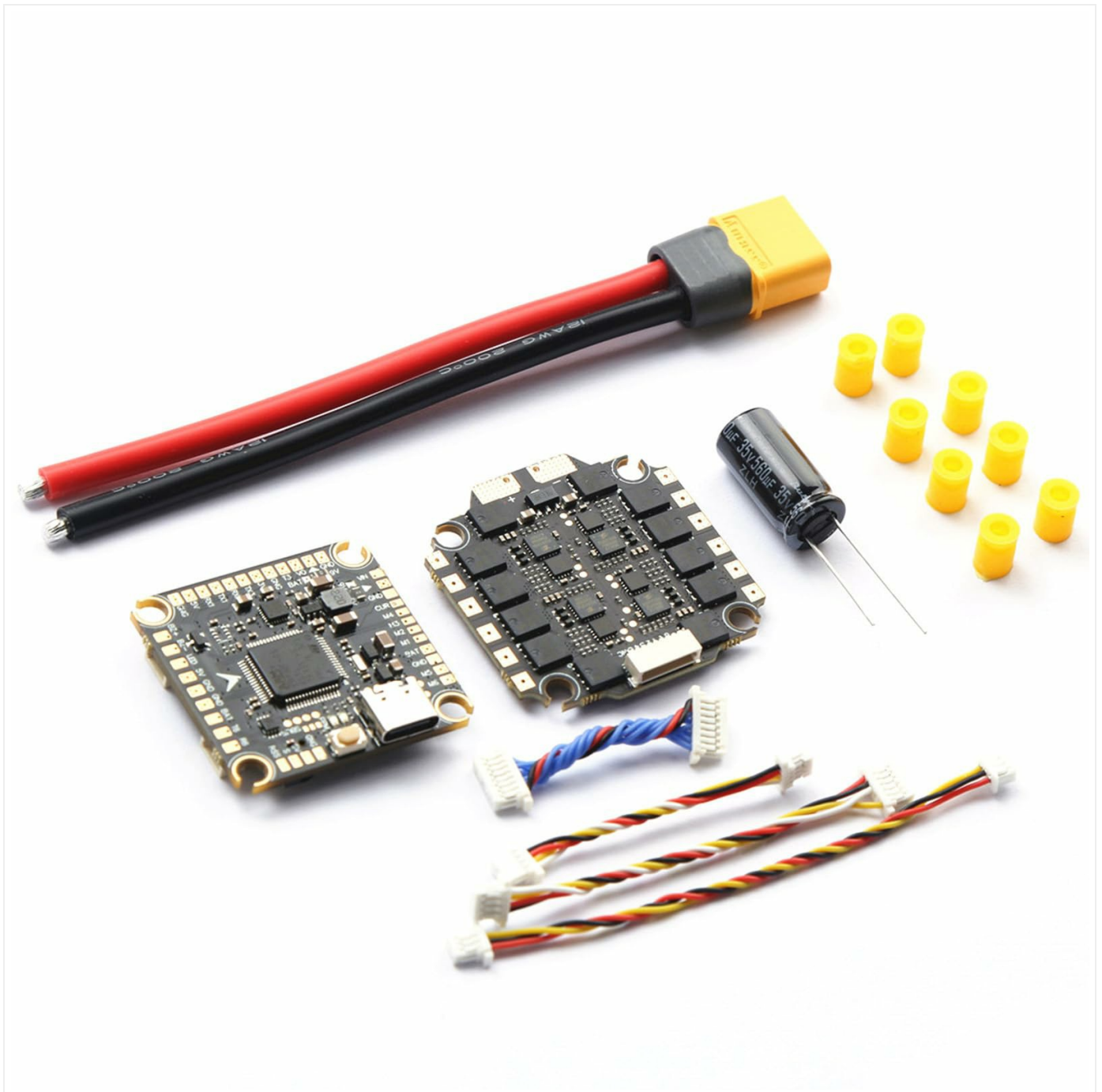
Image 1.1: The Goolsky Tracker F405 V2 Flight Control FC and BLS-65A 4-in-1 ESC Stack. This image displays the compact design of the flight controller and electronic speed controller unit, highlighting its integrated nature for FPV drone applications.
