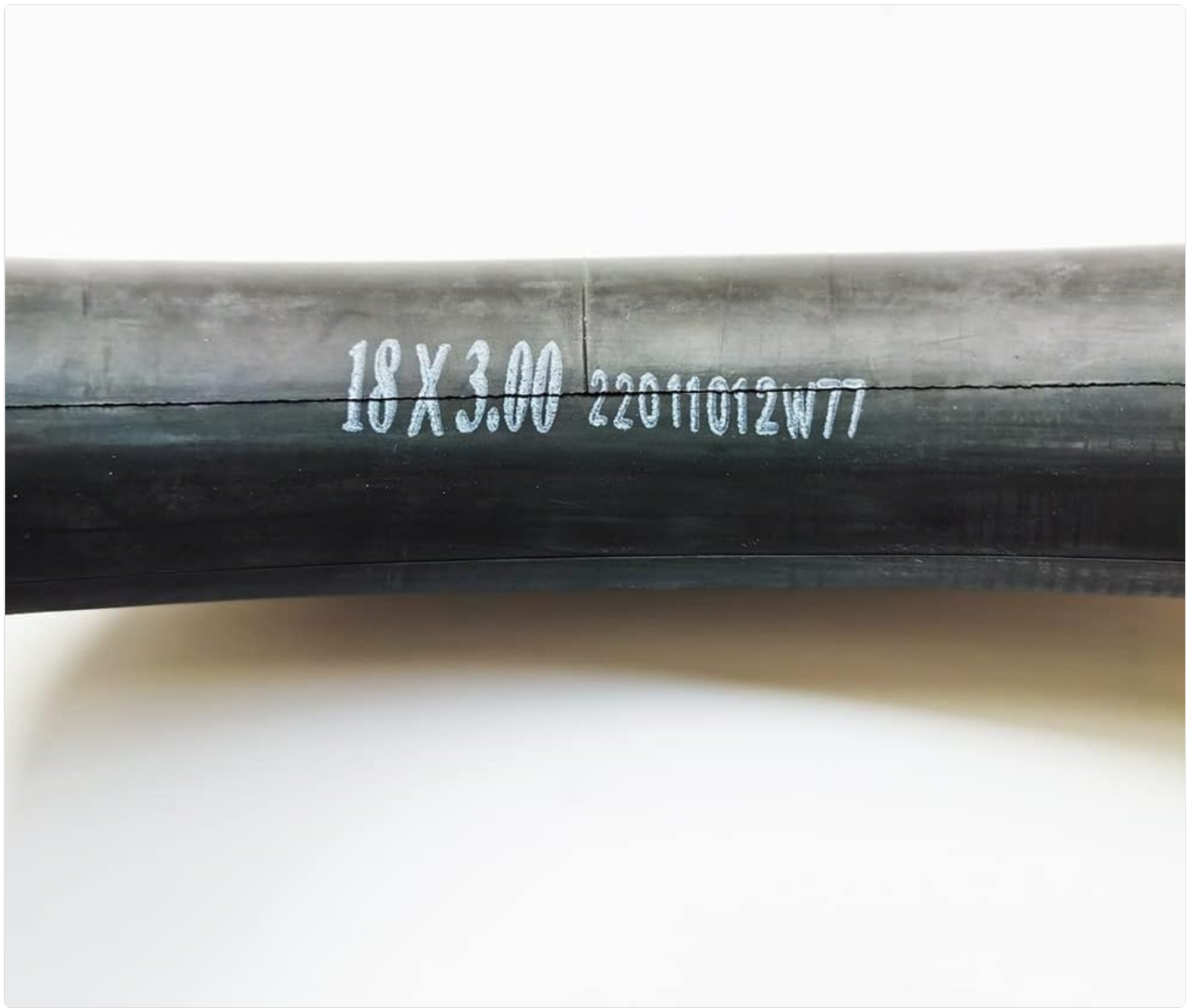
Image: Detail of the 18x3.00 size marking on the inner tube.
