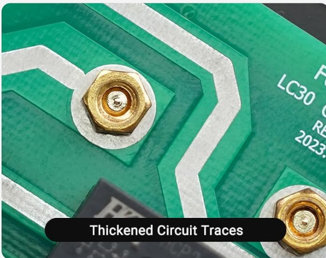
Figure 5: Close-up images of the LC30's superior quality components, including high-quality relays, 390Ω load resistors, thickened circuit traces, and user-friendly terminal design.
