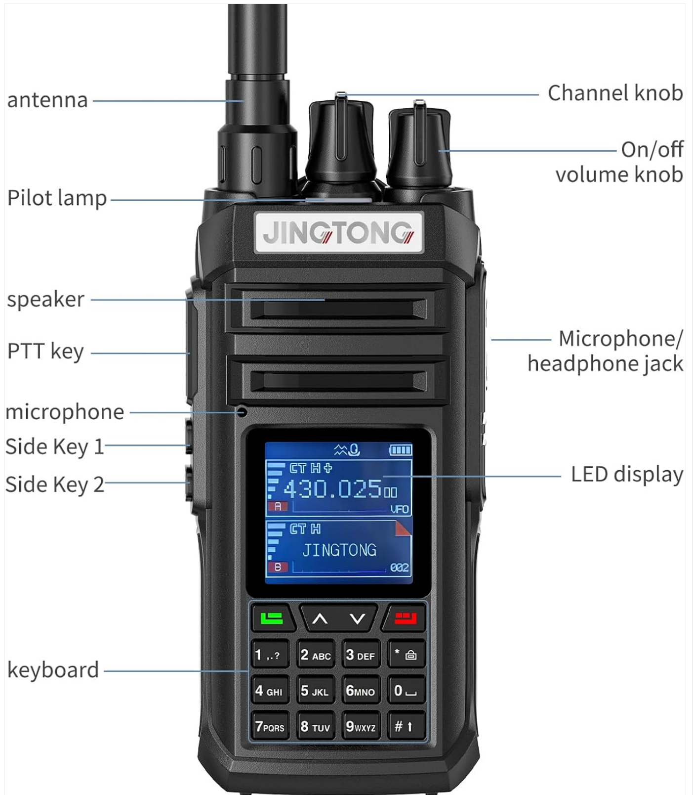
Image: Labeled diagram of the JINGTONG JT-3988 showing its main components and controls.
