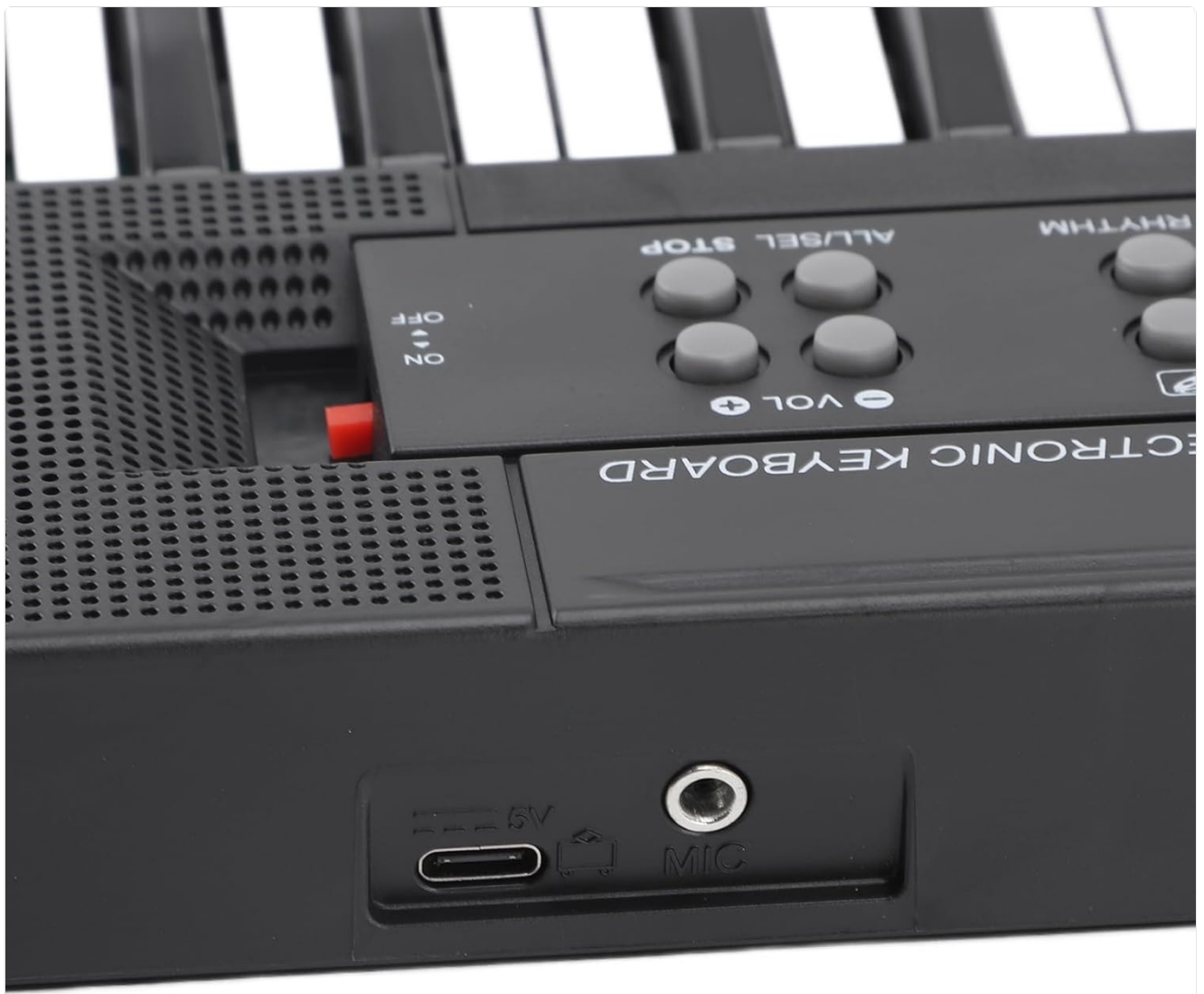
Image: A close-up view of the keyboard's side, showing the 5V USB power input and the microphone input jack.
