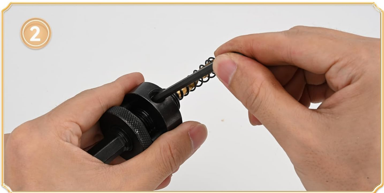
Image: Step-by-step visual guide for inserting the pilot drill and attaching the hole saw to the arbor.
