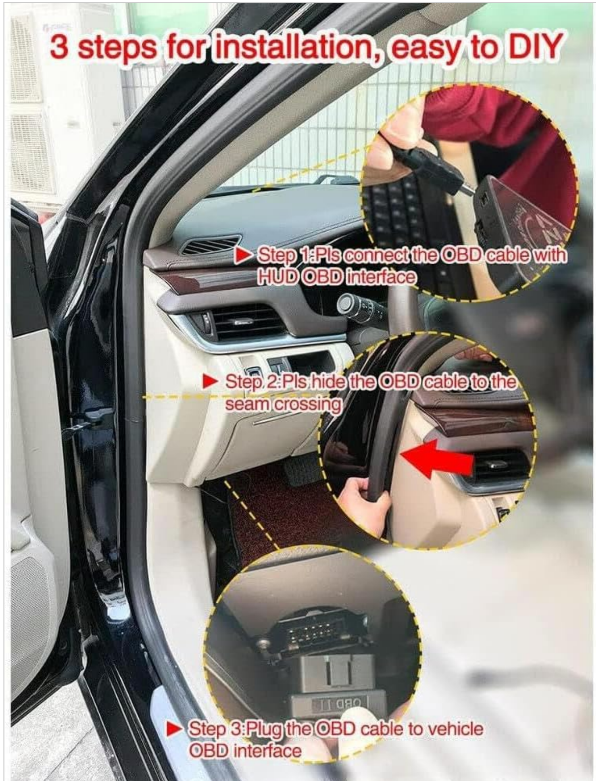
Three-step installation guide: connecting the OBD cable to the HUD, hiding the cable, and plugging the OBD cable into the
