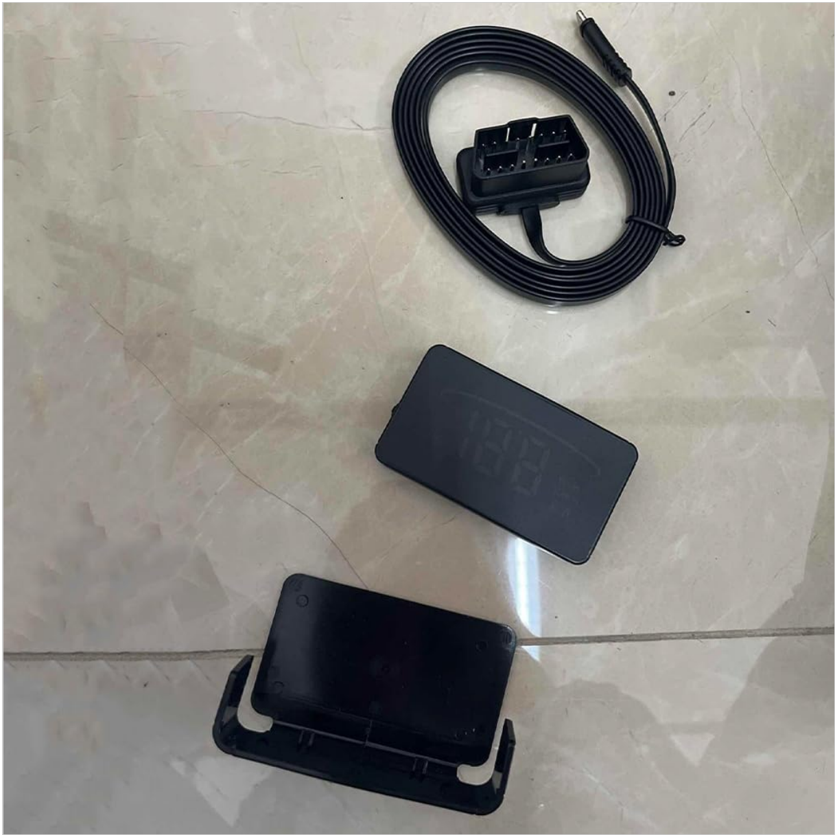
All components included in the package: the HUD unit, its hood, and the OBD cable.
