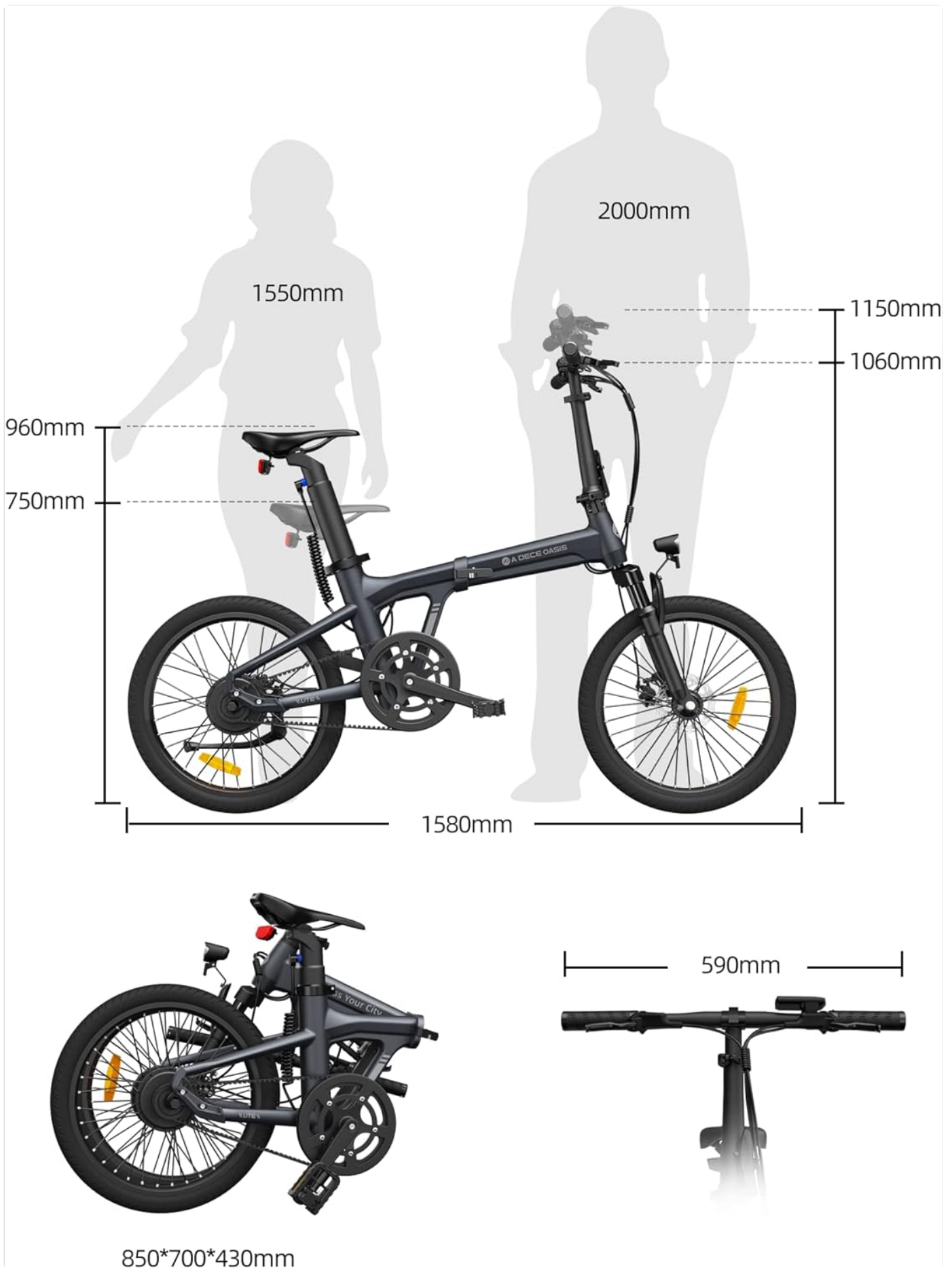
Figure 3.1: Unfolded and Folded Dimensions.
