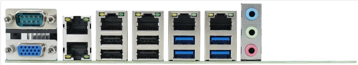
Figure 3: Detailed view of the rear I/O ports, including two VGA ports, six 2.5GbE Ethernet ports, USB ports, and audio jacks.
