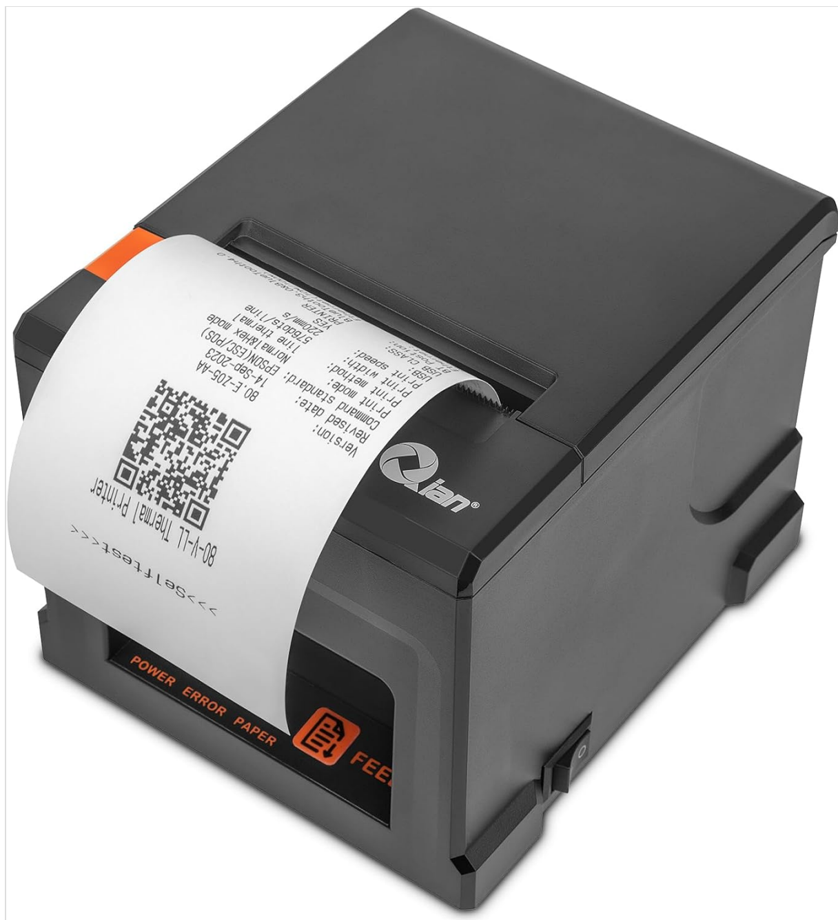
Image: Printer producing a self-test receipt, displaying printer information and QR code.
