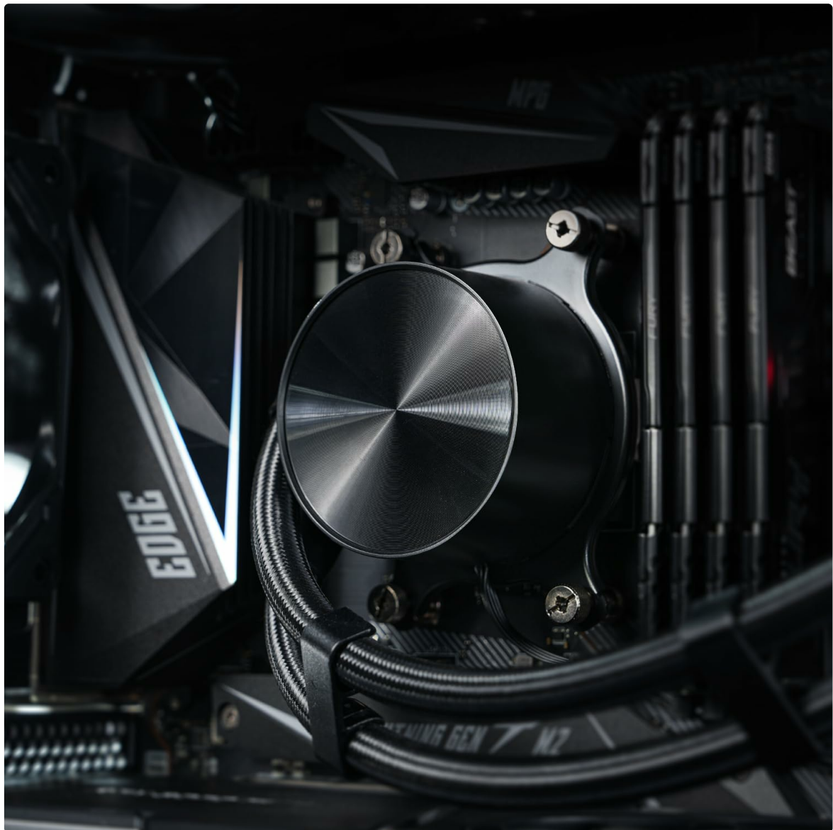
Image 4: The pump head of the FX360 PRO securely mounted on an AMD motherboard, illustrating the final installation step.
