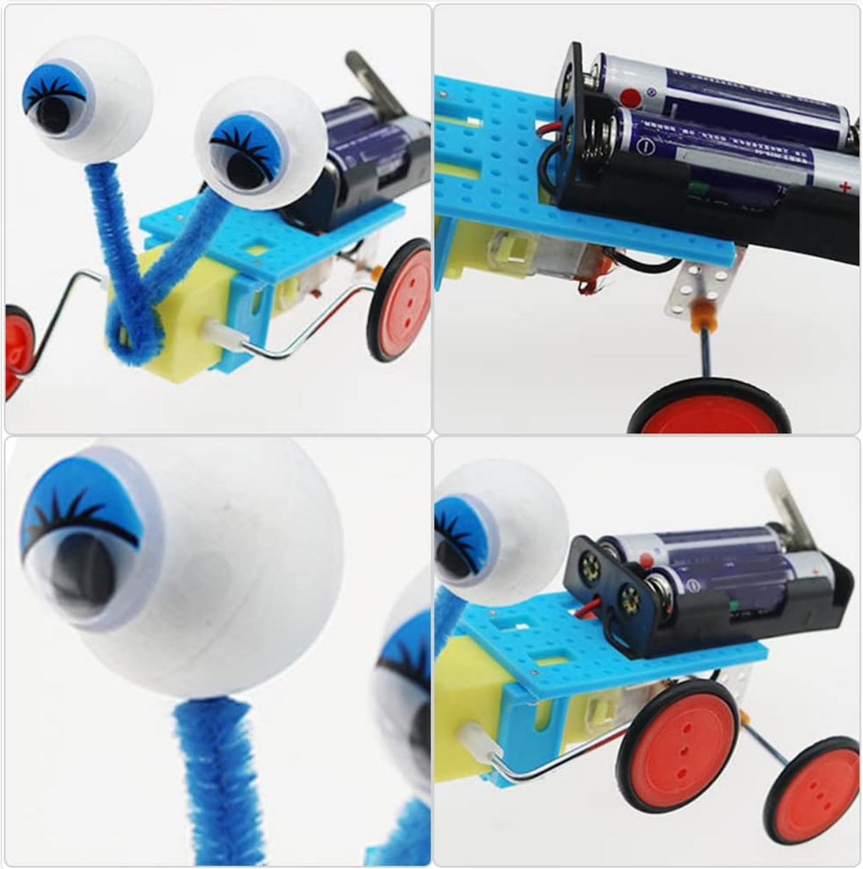
Image 3.1: Detailed view of the robot's internal components, including the battery box and motor, during assembly.
