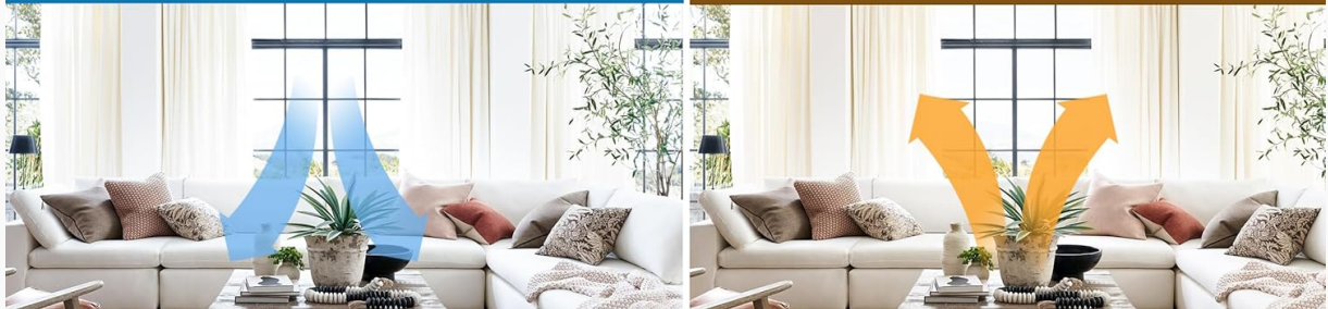
Figure 5.3: Visual explanation of the 6-speed reversible function, showing how airflow changes for summer (downdraft) and winter (updraft) modes.
