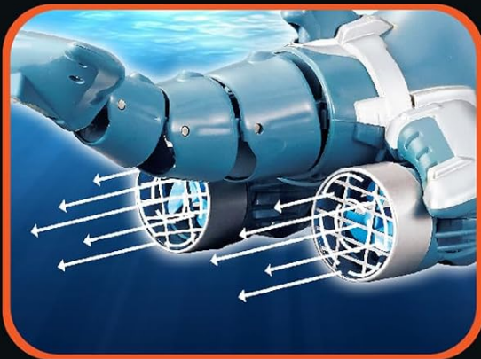
Figure 3: Detailed view of the dolphin boat's simulated tail movement, the mechanism for detaching the tail, and the double propeller drive system.
