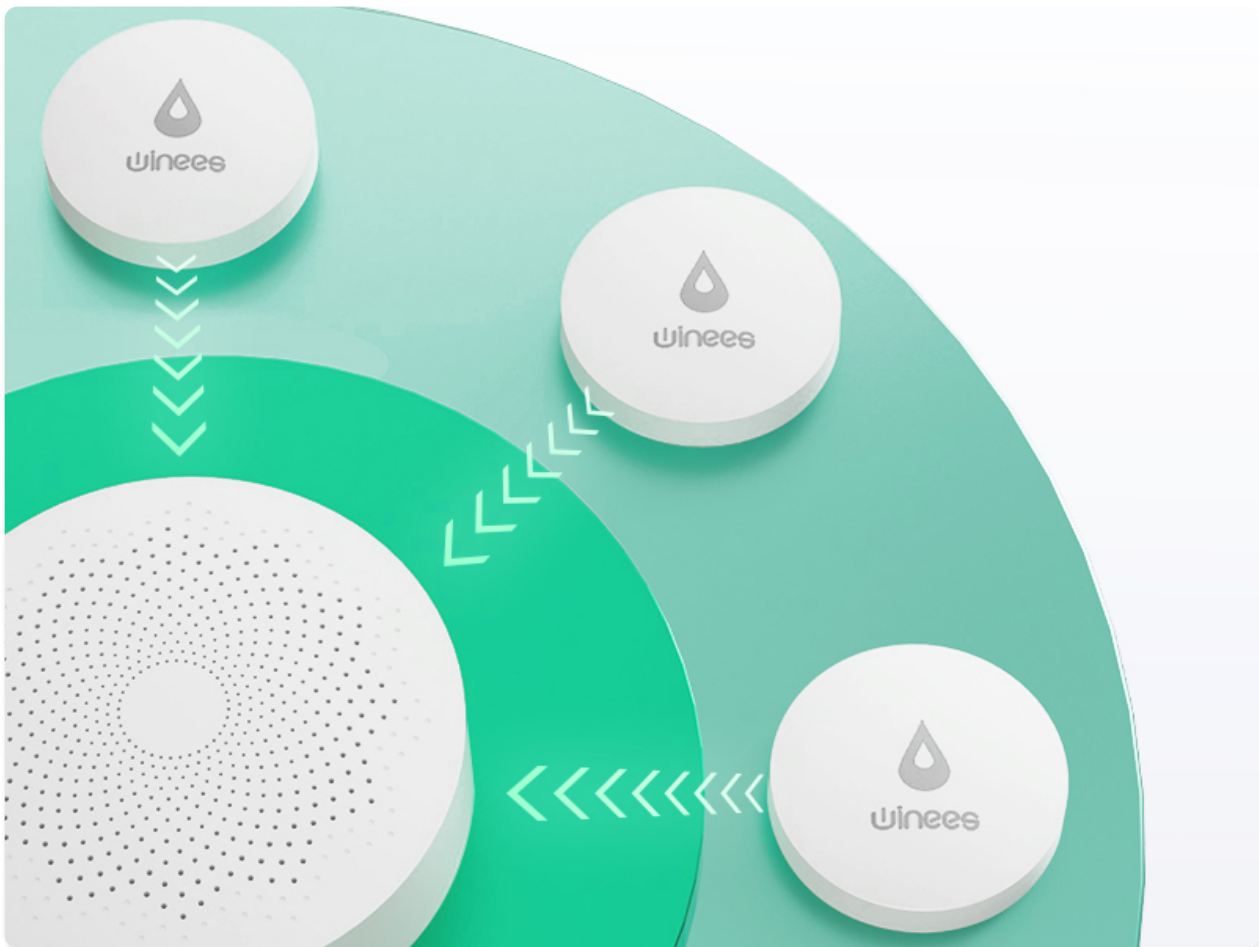
Image: Direct pre-pairing between the hub and sensor for simplified setup.
