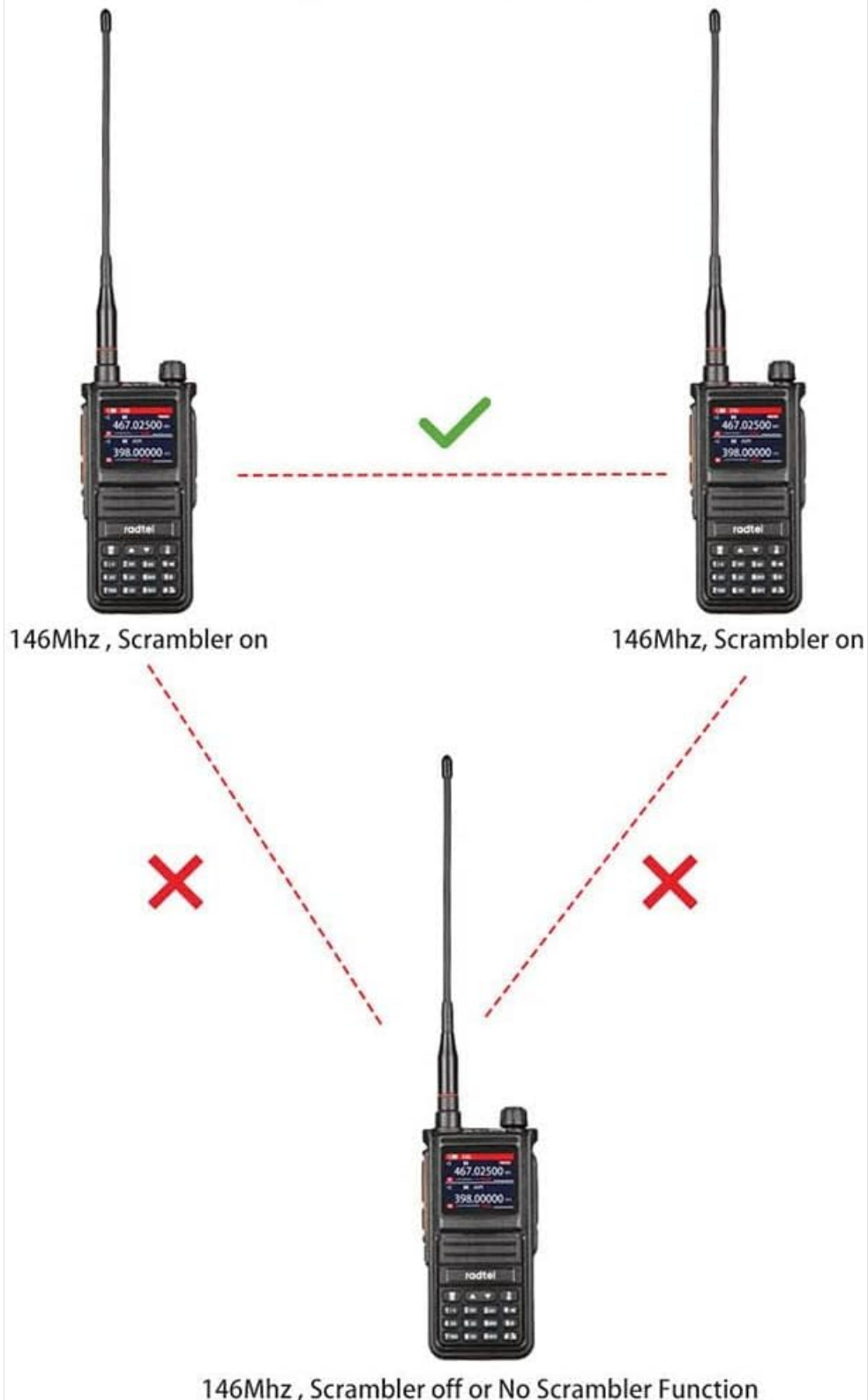
Figure 2.2: When activated, the voice scrambler function prevents unauthorized listening on the same frequency.
