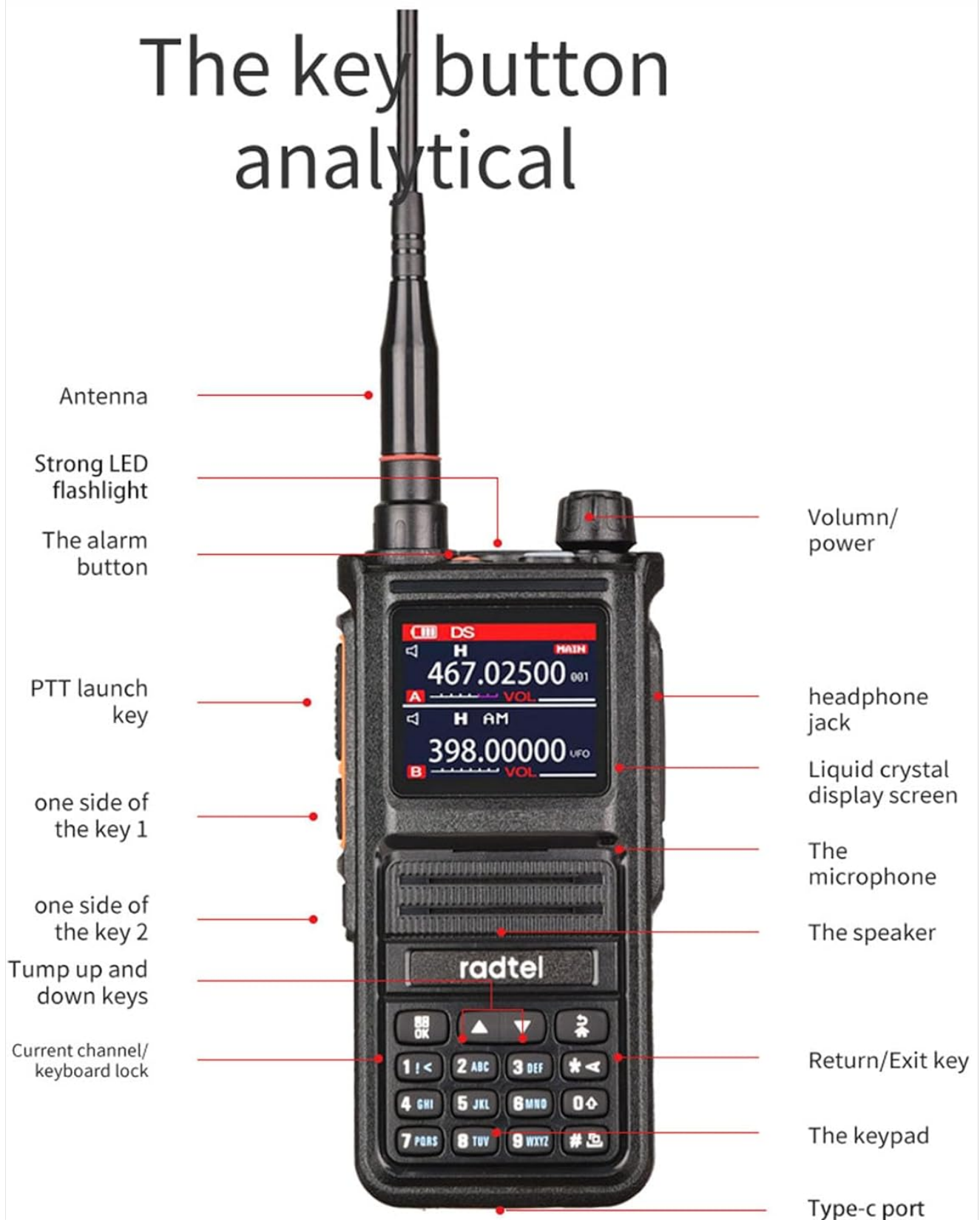
Figure 4.1: Front view of the Radtel RT-470X with key components labeled.
