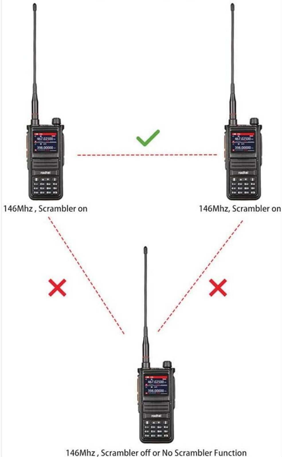
Figure 6.3: How the Voice Scrambler Function works.
