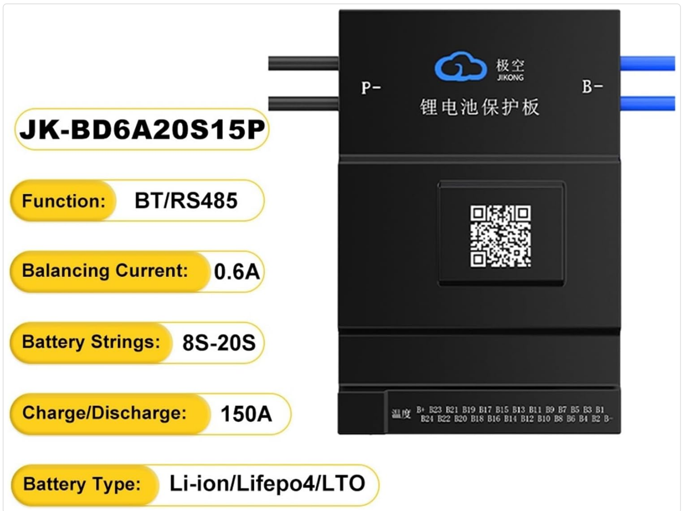
Image: JK Smart BMS BD6A20S15P highlighting its key features and specifications, including Bluetooth connectivity and active balancing.
