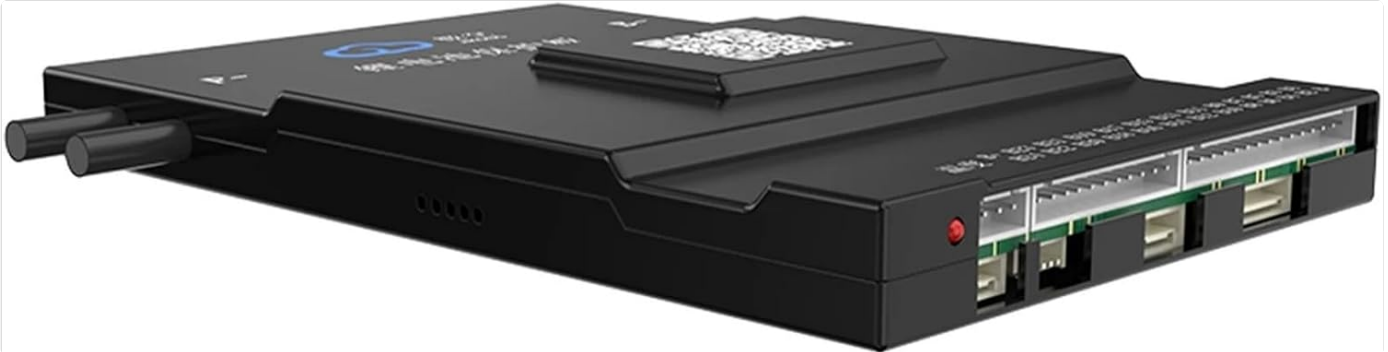
Figure 5.1: Side view of the BMS, illustrating the various connection ports for balance wires, temperature sensor, and other peripherals.
