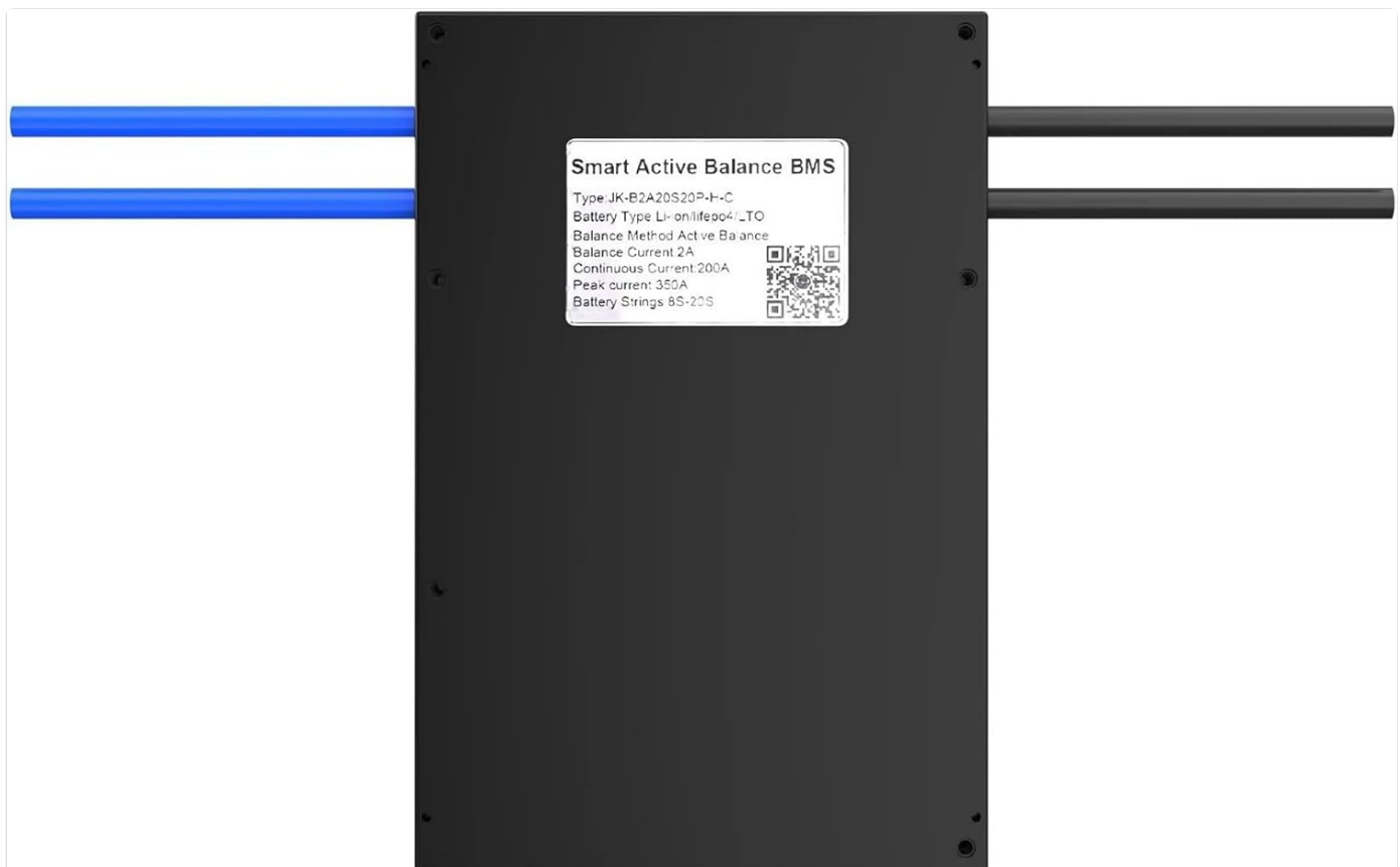
Figure 2.3: Rear view of the Smart Active Balance BMS, displaying the product label with model type (JK-B1A20S20P-C), battery type
