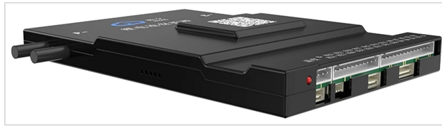
Image 5.3: Side profile of the BMS, providing a clear view of the balance wire interface and the robust construction.
