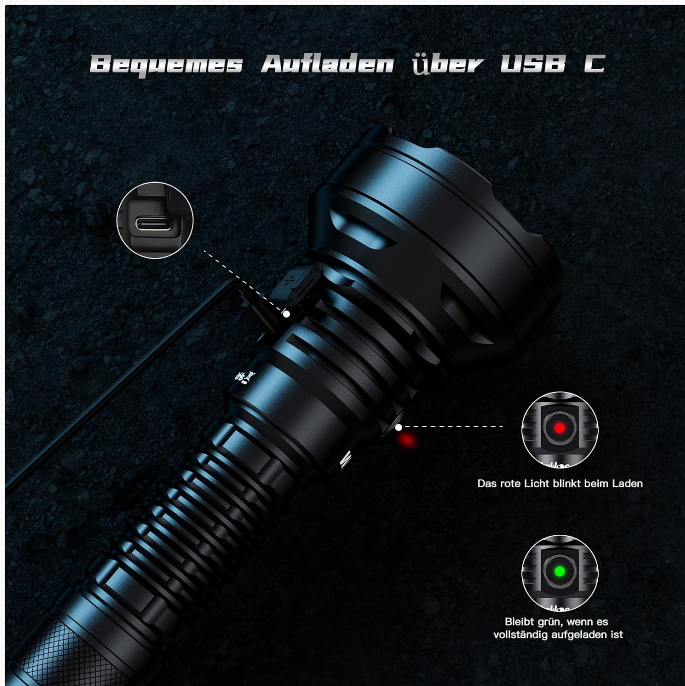
Image: The Wurkkos TD01C flashlight being charged via its USB-C port. The image highlights the charging cable connection and the red/green indicator lights that signal charging status.
