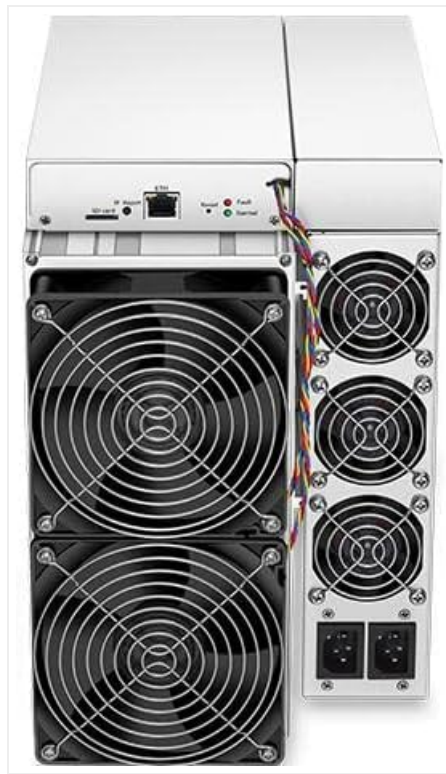
Figure 4.3: Rear view of the Antminer S19j XP, displaying the Ethernet port, indicator lights, and power input sockets, along with the exhaust fans.
