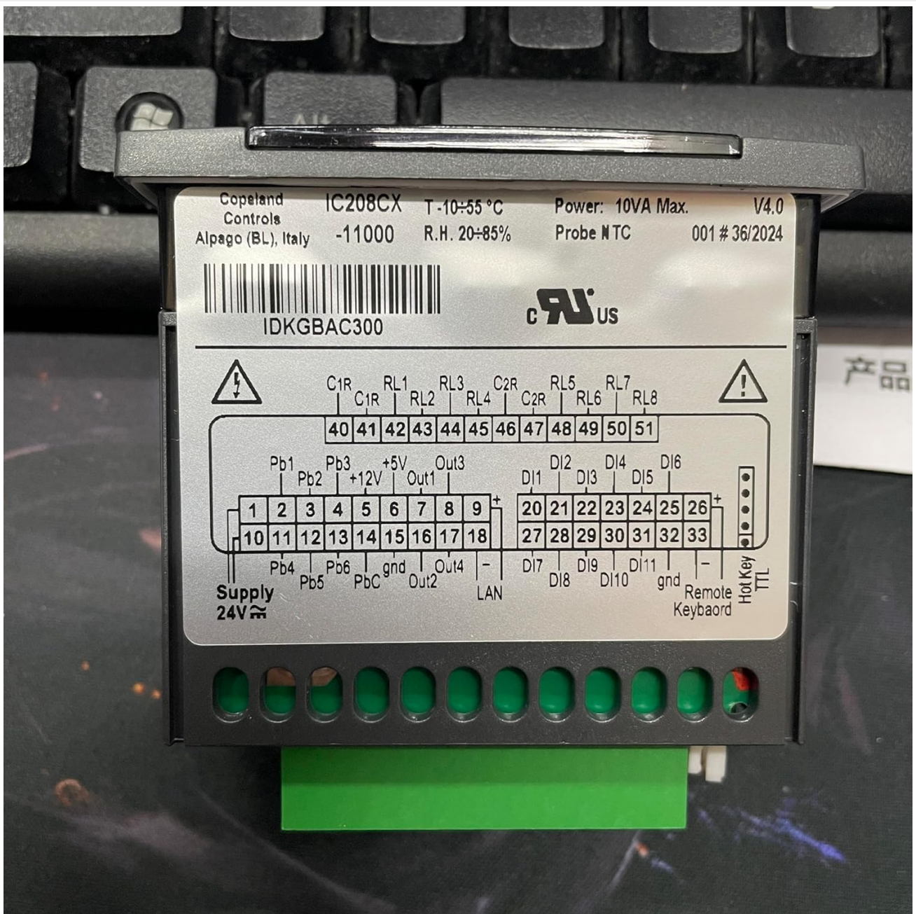
Figure 2: Rear view of the IC208CX-11000 controller, displaying the terminal block for electrical connections and detailed wiring labels. Note the model information "IC208CX -11000" and the Alapago (BL), Italy origin. A relevant link for further information is IDKGBAC300 .
