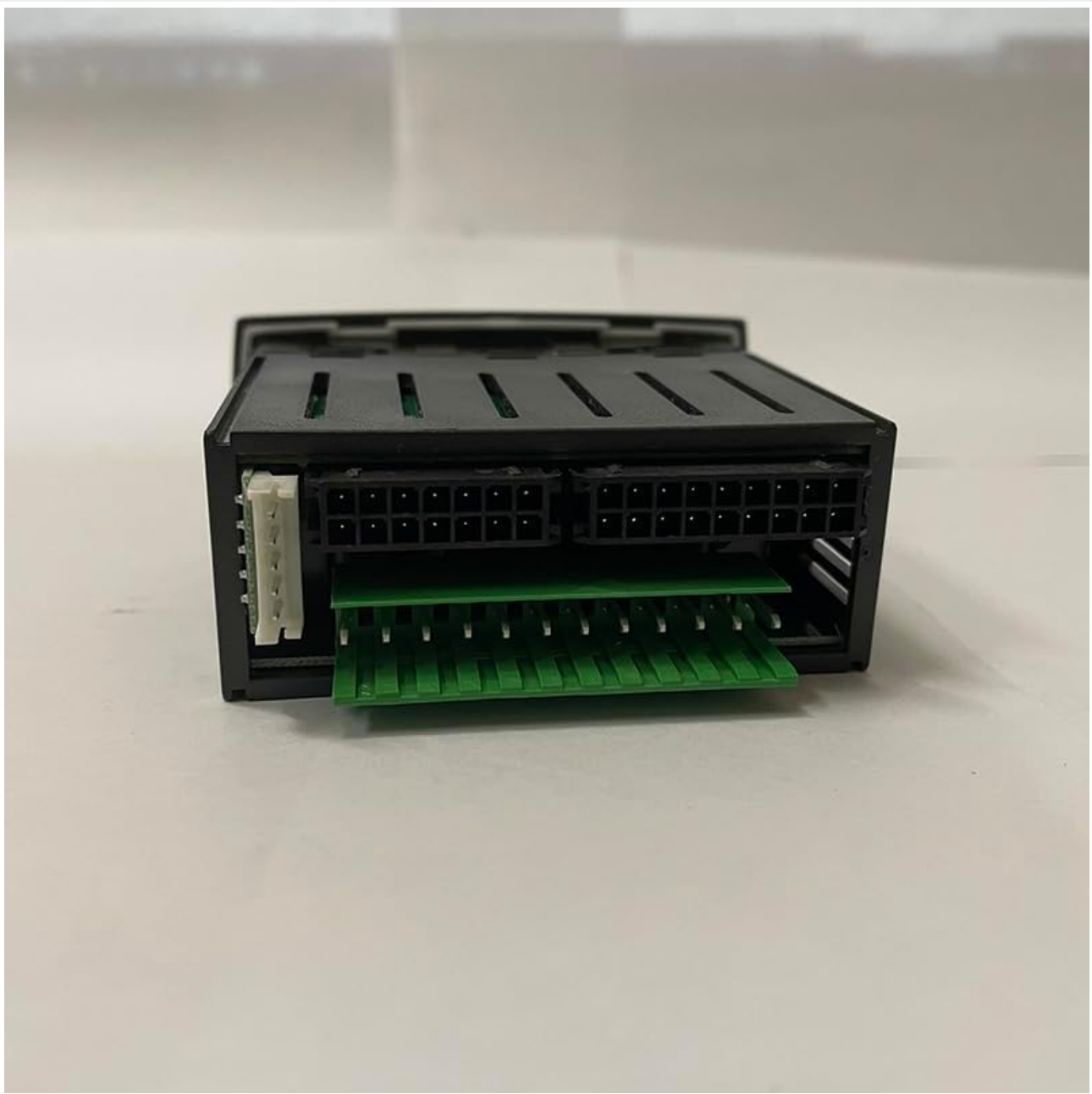
Figure 3: Side view of the IC208CX-11000 controller, illustrating the various connector ports for external modules or accessories.
